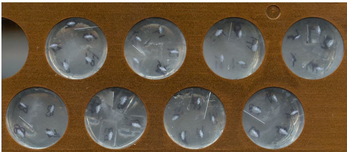
Figure 60. Photograph of whole mounted Sand Flathead otoliths prepared for LA-ICP-MS using the protocol developed here. Otoliths of similar sizes were embedded together and polished to expose the individual centra.
