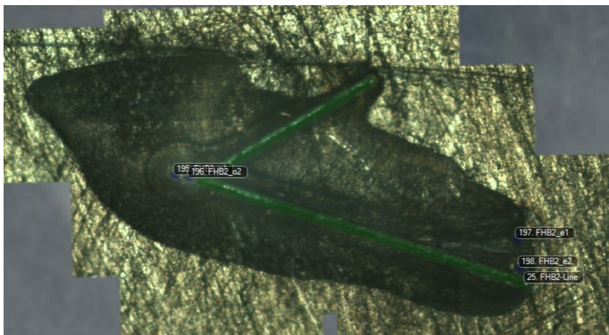
Figure 61. Example of laser ablation transects across the otolith surface from the point of natal origin to the edge (capture) across different axes.
